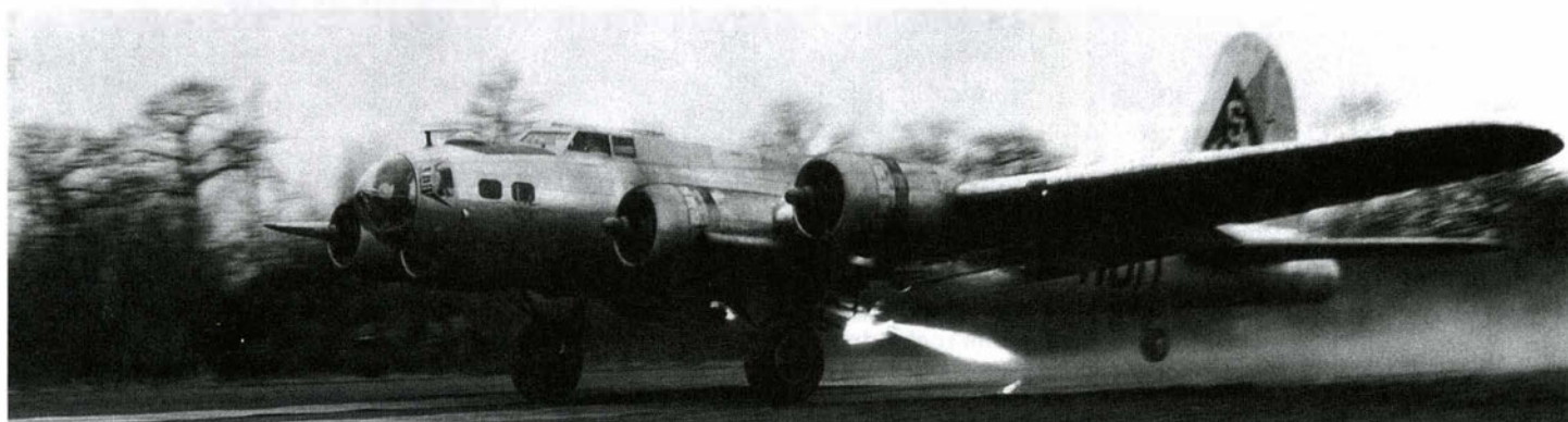
1. First rocket fires and tail lifts. Note replaced tail with "S" marking.
